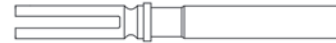
57 Socket, straight, crimp removable (20-22 awg) 58 Socket, straight, crimp removable (24-26 awg) 59 Socket, straight, crimp removable (28-30 awg)
