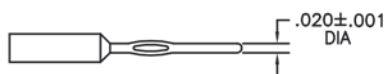
64 Socket, straight, press-fit, .203" (Board: .093"-.125") 65 Socket, straight, press-fit, .323" (Board: .156"-.200") 66 Socket, straight, press-fit, .403" (Board: .250 or <)
