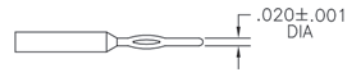
87 Socket, straight, press-fit, .188" (Board: .093"-.125") 88 Socket, straight, press-fit, .308" (Board: .156"-.200") 89 Socket, straight, press-fit, .388" (Board: .250 or <)
